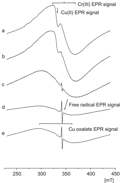
Fig. 1. EPR spectra of CCB treated wood exposed to (a) *G. trabeum*, (b) *P. monticola*, (c) *A. vaillantii*, (d) and *L. pinastri* (e) for eight weeks.
