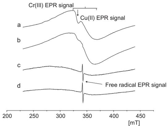
Fig. 2. EPR spectra of CCB treated wood acidified with (a) 1%, (b), 5% (c) and 10% (d) aqueous solution of oxalic acid.
