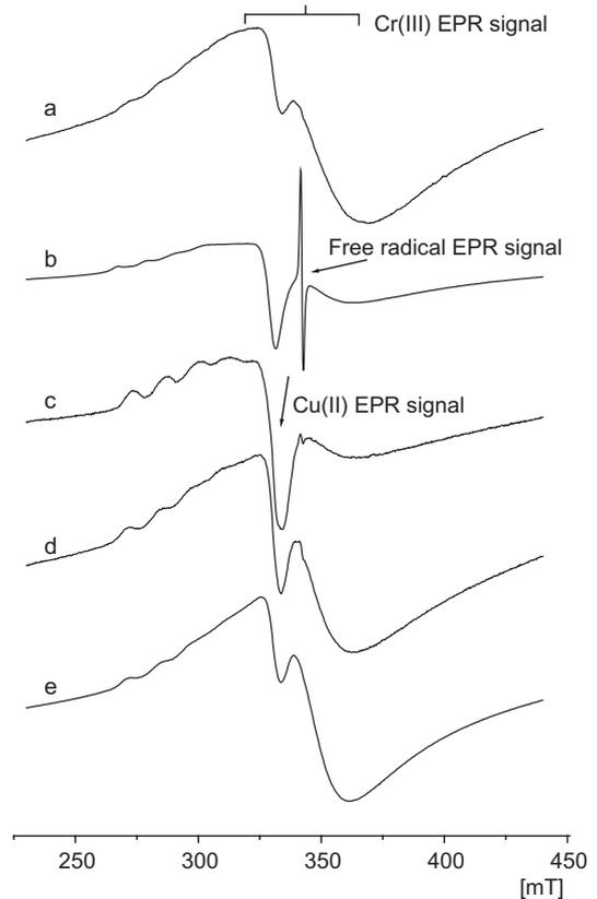
Fig. 3. EPR spectra of CCB treated wood acidified with (a) 5%, aqueous solution of sulfuric (b), lactic (c), formic (d) and acetic acid (e).
