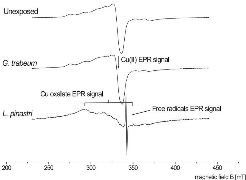
Fig. 2: EPR spectra of Tanalith E treated samples unexposed and exposed to brown rot fungi *Gloeophyllum trabeum* and *Leucogyrophana pinastri* for 16 weeks.
