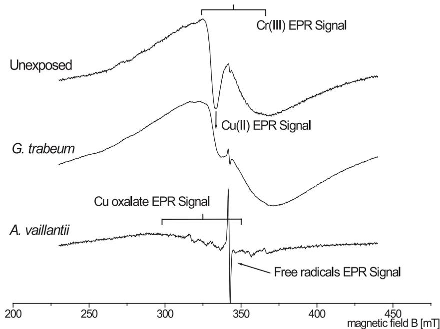
Fig. 1: EPR spectra of CCA treated samples unexposed and exposed to brown rot fungi *Gloeophyllum trabeum* and *Antrodia vaillantii* for 16 weeks.
